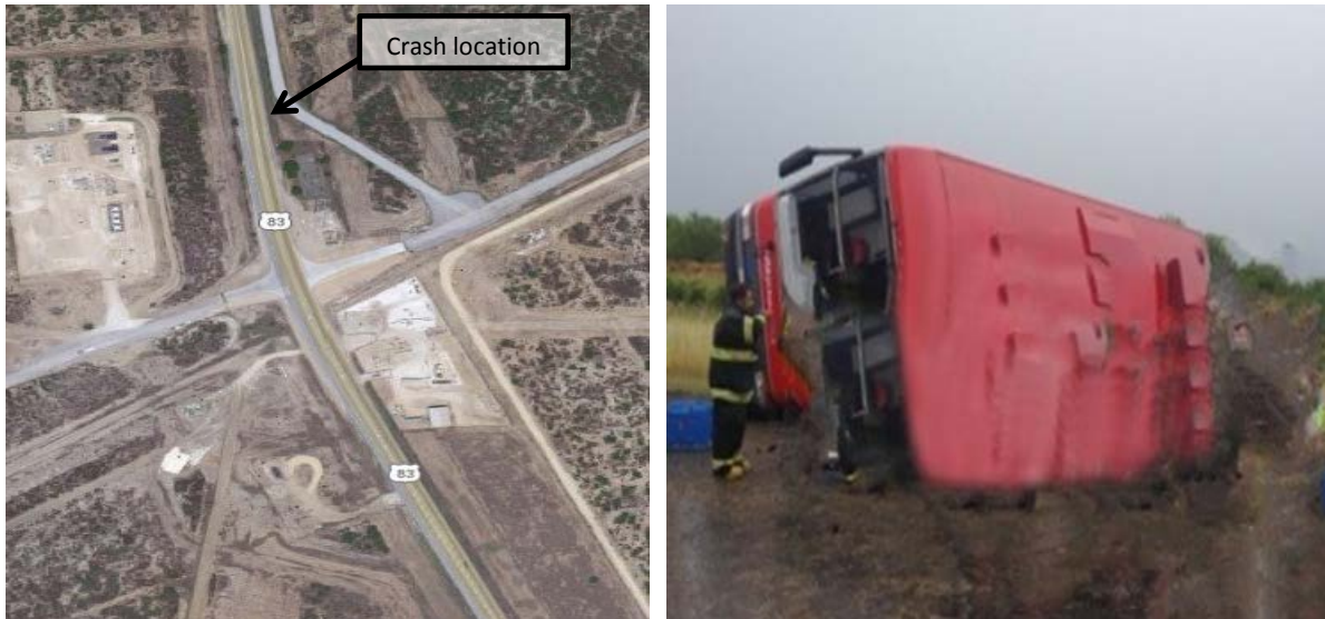
Figure 1. The photograph on the left shows an aerial view of US-83 showing the crash location and the horizontal alignment of the roadway. The photograph on the right shows the final rest position of the motorcoach on its left side.
