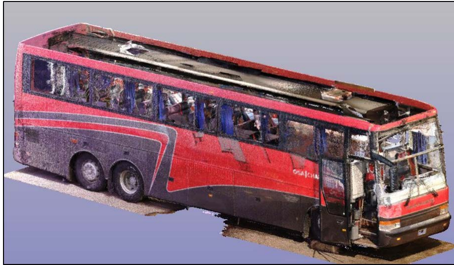
Figure 2, 3D scanned image of the right side damage to the 1998 Van Hool motorcoach.
