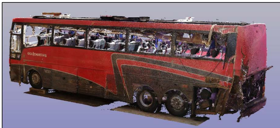
Figure 3, 3D scanned image of the left side damage to the 1998 Van Hool motorcoach.
